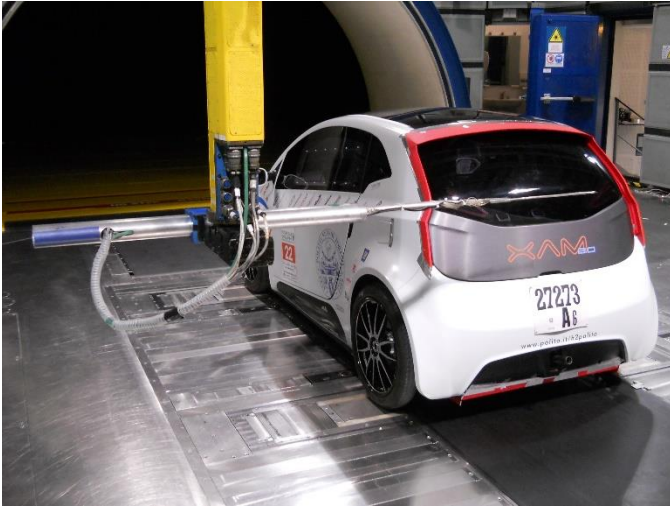
Figure 5 - Pressure field measurement with 14-holes probe
