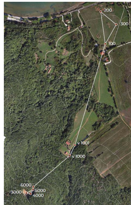
Fig.2. Topographic network overlaying the orthophoto generated by the fixed wing UAV flight
