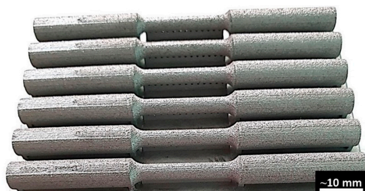
Figure A1. Image of some produced tensile specimens on the building platform of 90 \times 90 \text{ mm}^2 .
