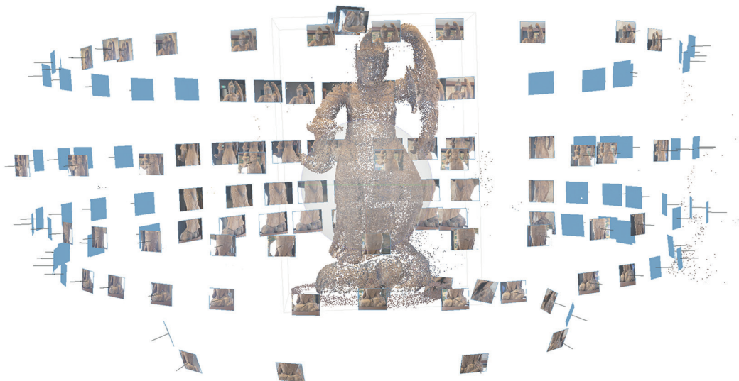
Fig. 4. Photo alignment with sparse cloud (photos by F. Ronco and S. Tamantini).
