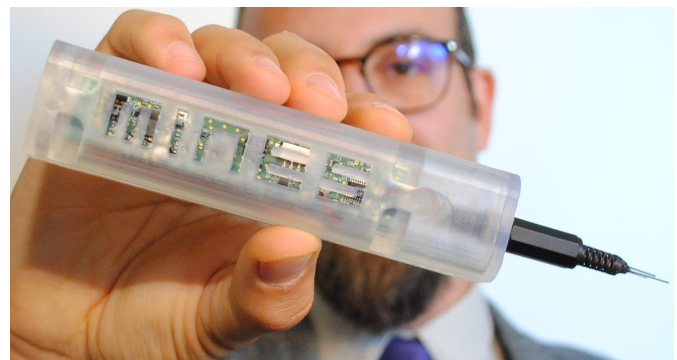
Fig. 1. The smart pen for direct and continuous classification of anaesthetics in human serum.
