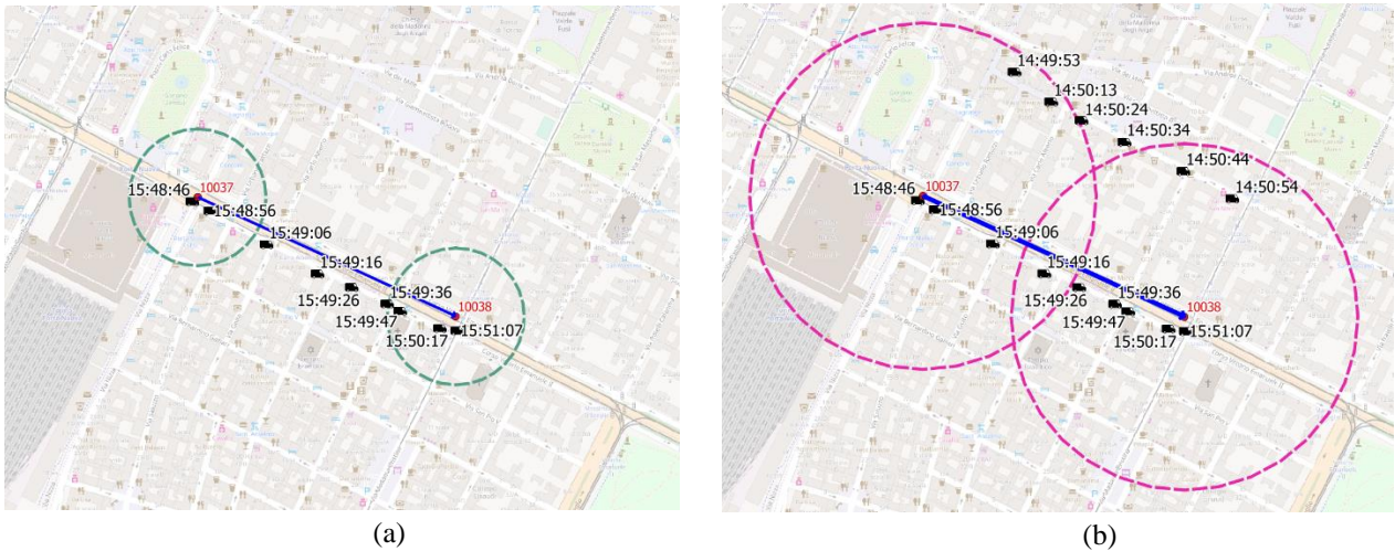
300 Fig. 6 Example of a link (blue line) connecting nodes 10037 and 10038, both representing intersections of two “Road2lanes” in the city centre. The 301 images represent two possible radii length: (a) 100 m and (b) 250 m (Source: QGIS).
