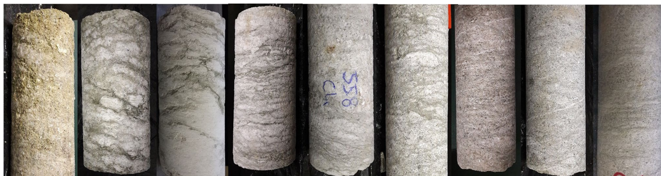
Fig. 2 Samples of branching selenite gypsum, underlining the mesoscopic heterogeneity of the material
