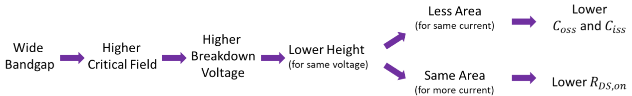
Figure 5 Relation between material properties and the characteristic of the components for vertical devices.
