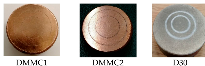
Figure 9. Wear scars on disks after test.
