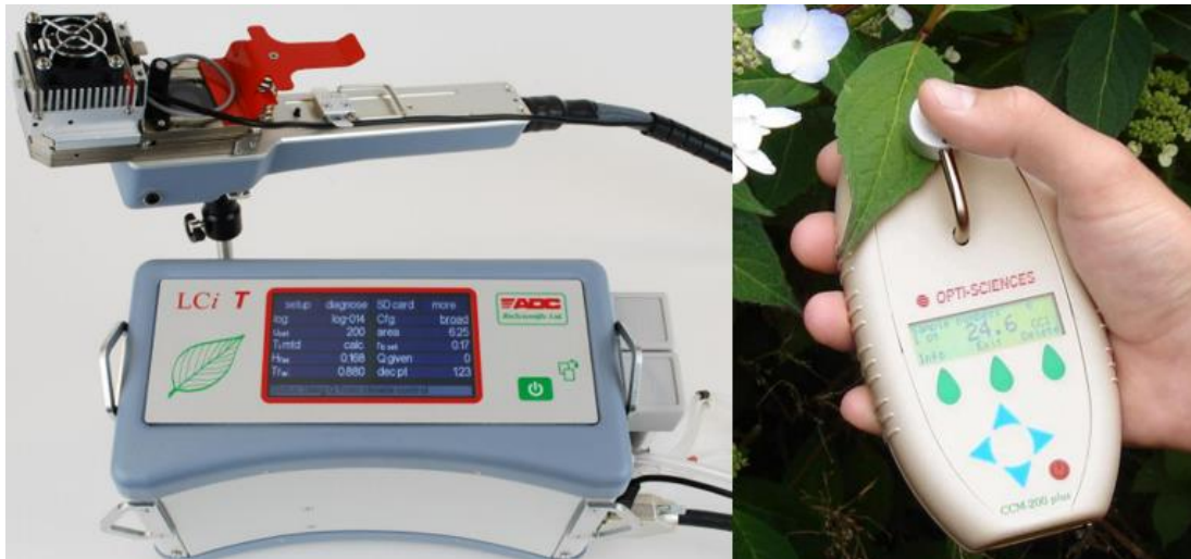
Figure 6. On the left side the Infrared Gas Analyzer (IRGA); On the right side the Chlorophyll Content Meter (CCM-200).
