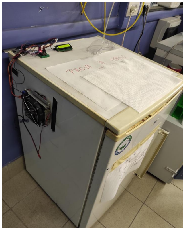
Figure 16. The climatic chamber used in this experiment.
