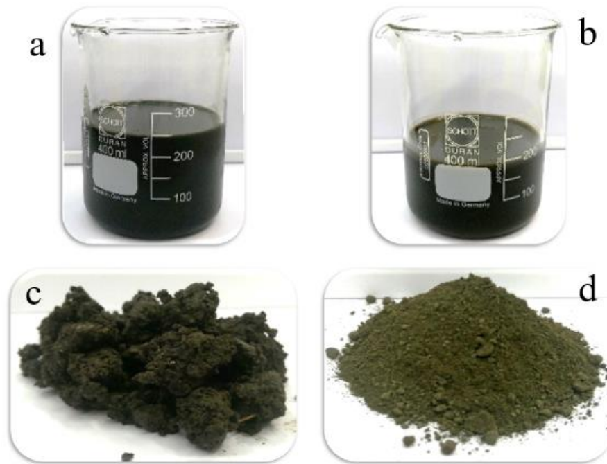
Figure 4. The four SSADs used in this work. a: primary SSAD; b: secondary SSAD; c: centrifuged SSAD; d: dried SSAD.
