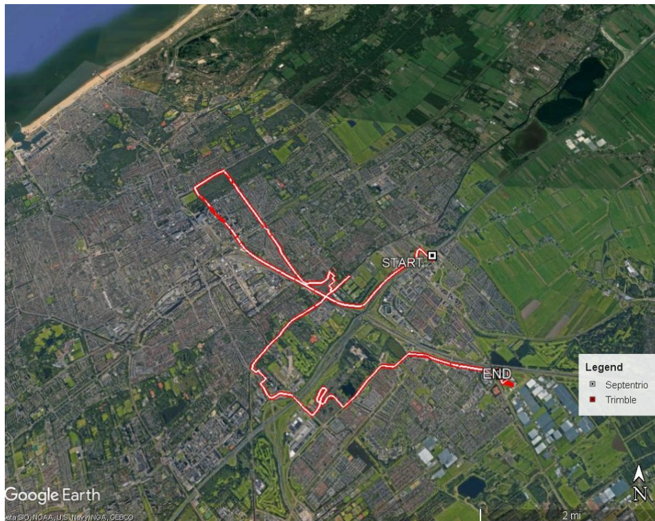
Figure 5.21: The Google Earth trajectory of the collected GNSS raw data using a car equipped with GNSS antenna, front-end (USRP N210) and commercial GNSS receivers (Septentrio and Trimble) in The Hague, The Netherlands.
