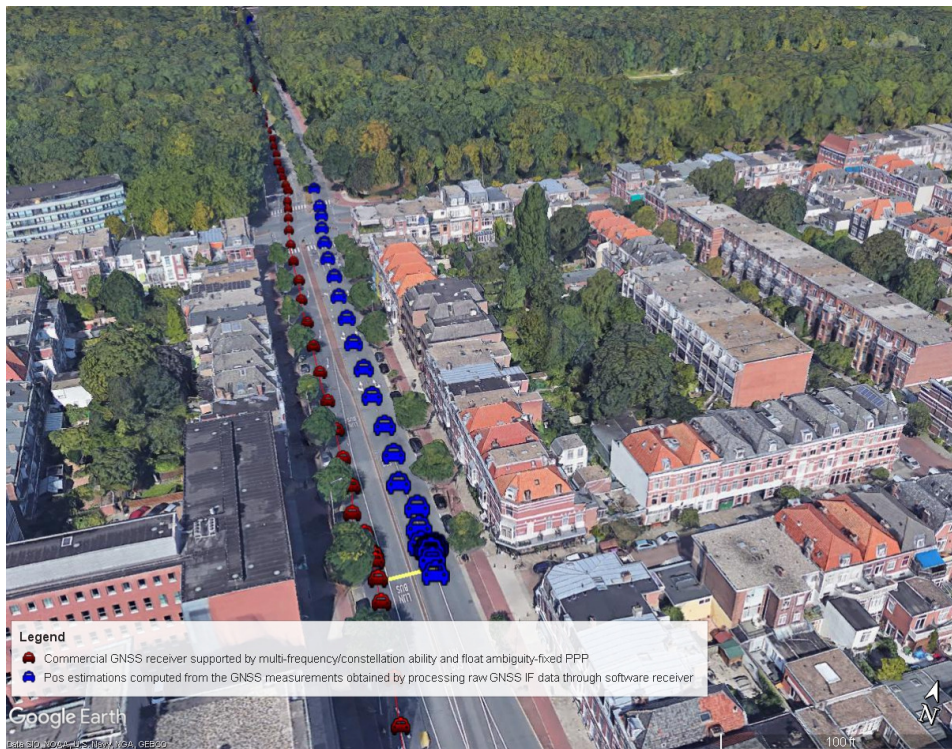
Figure 5.22: Biased position estimation due to the multipath effect and/or NLOS reception.
