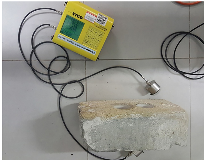
Figure 4. Ultrasonic test setup.
