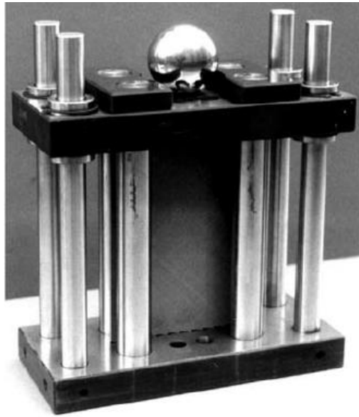
Figure 2.6: First ever anti-buckling fixture to test flat composite plates; Developed at NASA (41)
