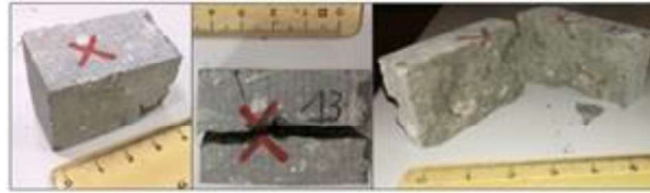
Figure 5. A melange specimen regularized by means of the diamond band saw for the PLT.
