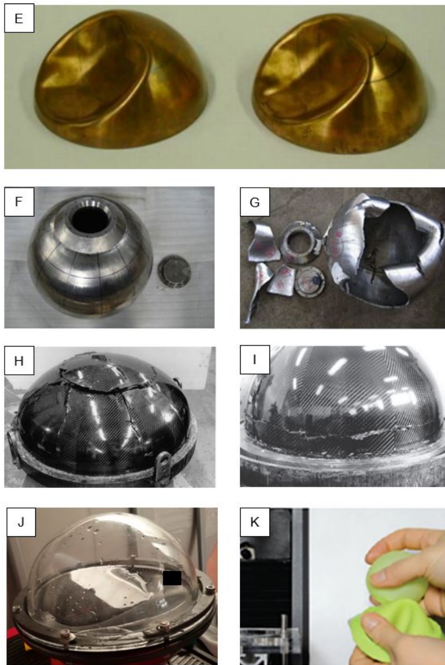
Figure 4.3: Experimental activities on spherical shells undergoing external pressure loading - examples of buckling failures: E) buckled copper-steel-copper hemispheres, manufactured by spinning [80], F-G) Ti6Al4V pressure hull before and after testing [81], H-I) Carbon Fiber Reinforced Polymer hemisphere after testing, J) failure of a Poly Methyl Metacrylate dome [82], K) manufacturing of almost-perfect Vinylpolysiloxane hemispheres [83]
