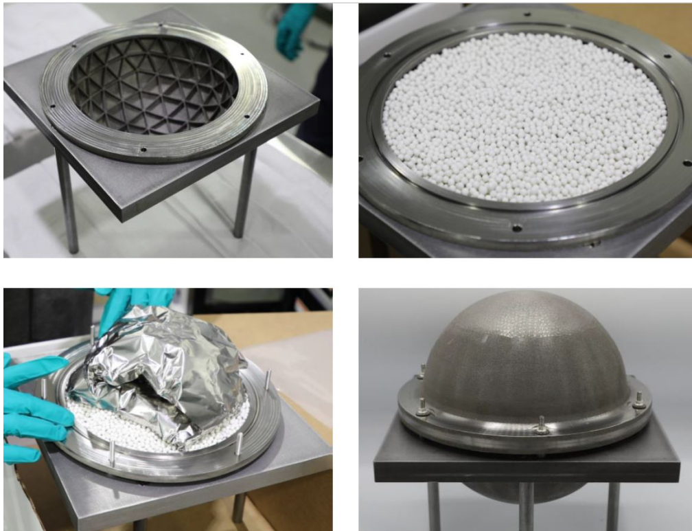
Figure 6.14: Relative environment test: test article preparation
