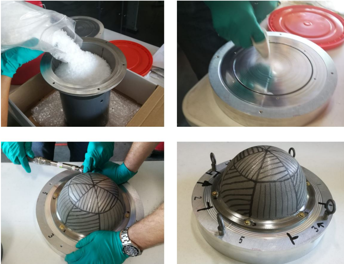
Figure 6.7: Hydrostatic test: test article preparation
