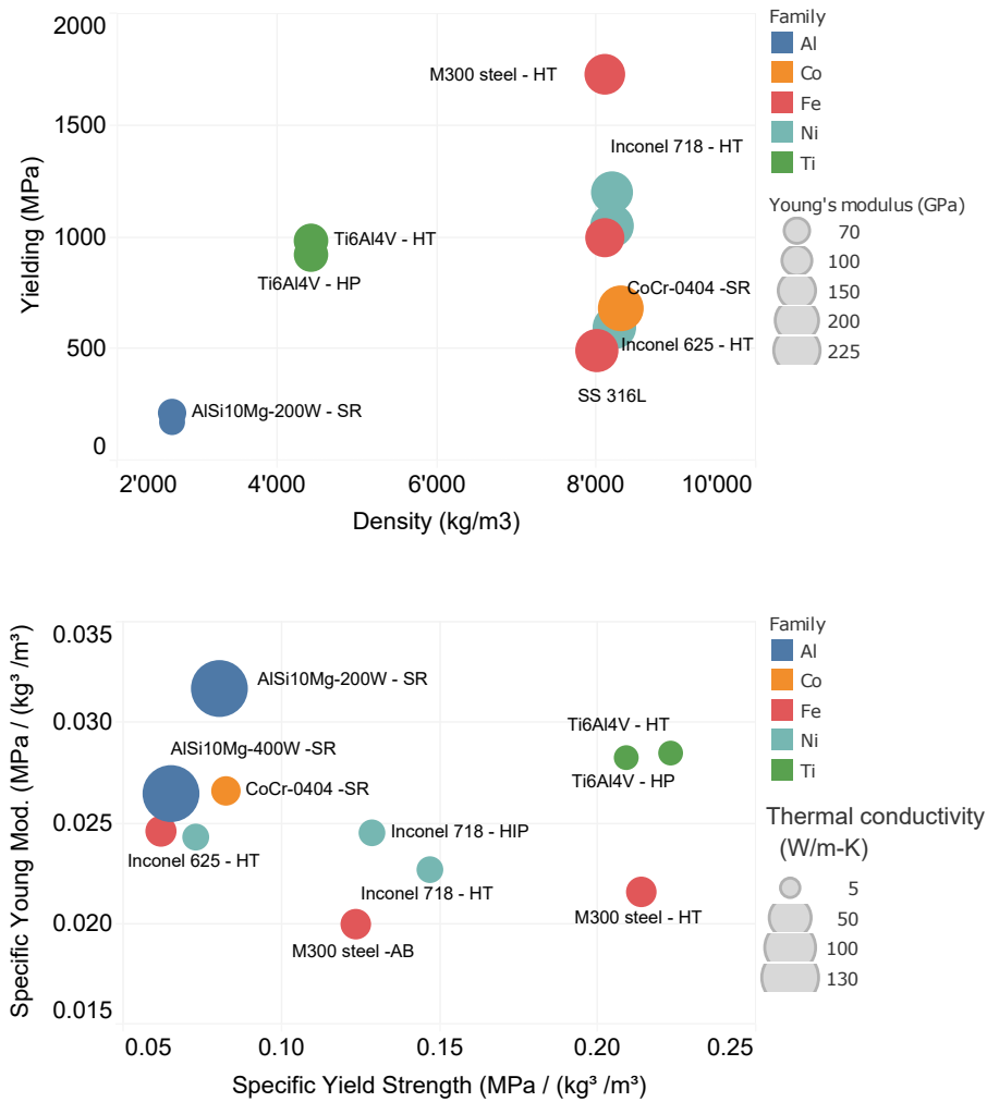
Figure 1.7: Examples of Ashby plot for material trade-off activities - alloys currently available for AM
