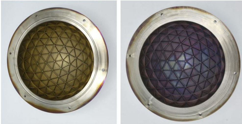
Figure 6.17: Component after testing: external surface, damaged ceramic beads, oxidized bottom and top hemispheres.
