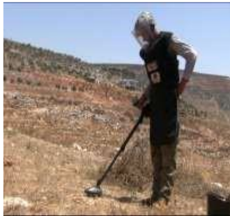
Figure 2 Landmine detection using metal detector
