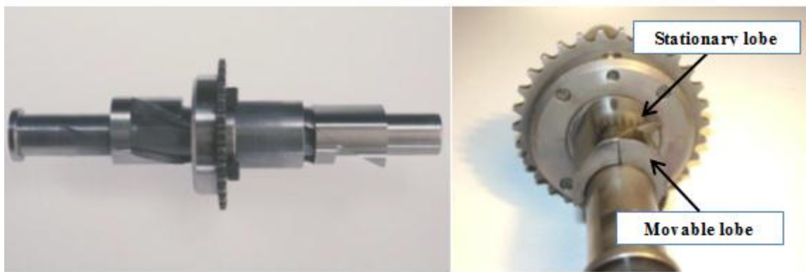
Figure 2.1. A prototype helical camshaft with the camshaft [1]
