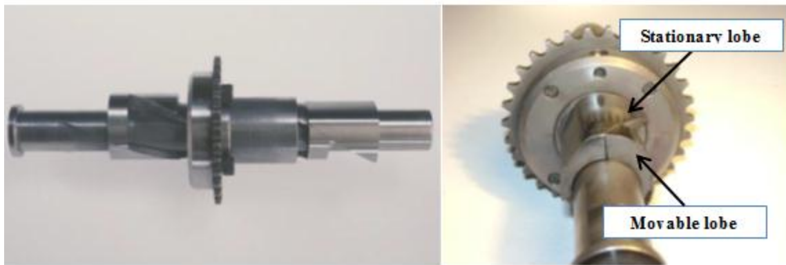
Figure 2.1. A prototype helical camshaft with the camshaft [1]
