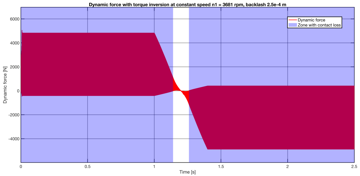
Figure 13. Dynamic force during torque inversion at resonance, n_2 region
