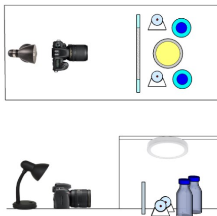
Figure 71) Schematics of the entire the experimental set-up, lamp and light images does not correspond to the actual equipment and only represents their placement.
