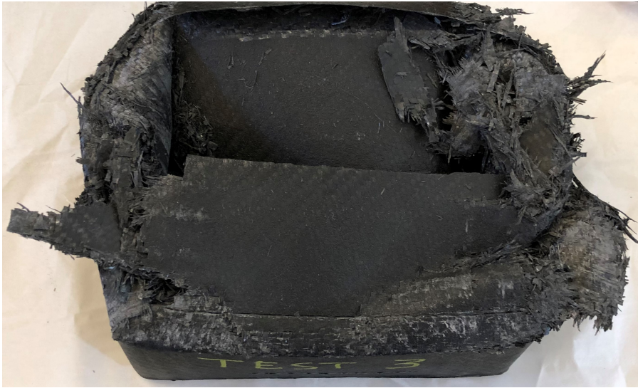
Fig. 4.27 Crushed CFRP component after impact with mass 300 kg and velocity 7.77 m/s.
