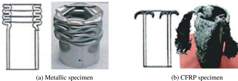
Fig. 2.2 Schematic drawings and real pictures of two different specimens after crush tests demonstrating differences in their energy absorption mechanisms [15].
