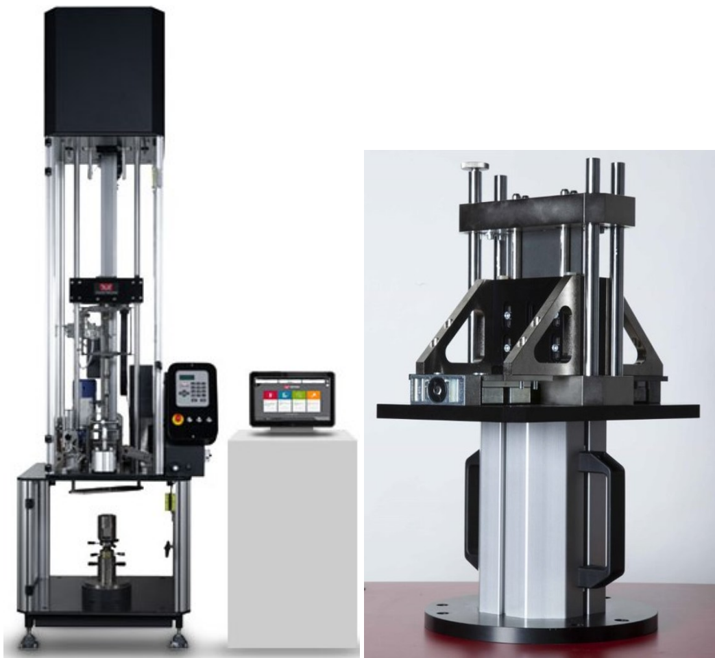
(a) Instron 9400 Series Impact Drop Tower [101] (b) Newly developed anti-buckling fixture.
