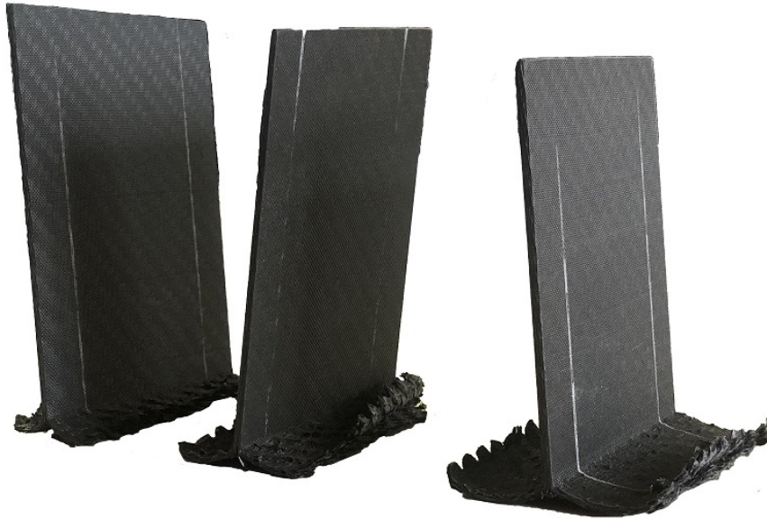
Fig. 4.11 Samples crushed with impact velocity of 4.69\text{ m/s} and different impact masses. From left to right impact masses were: 34\text{ kg} ( 375\text{ J} ), 50\text{ kg} ( 550\text{ J} ), and 70\text{ kg} ( 770\text{ J} ).
