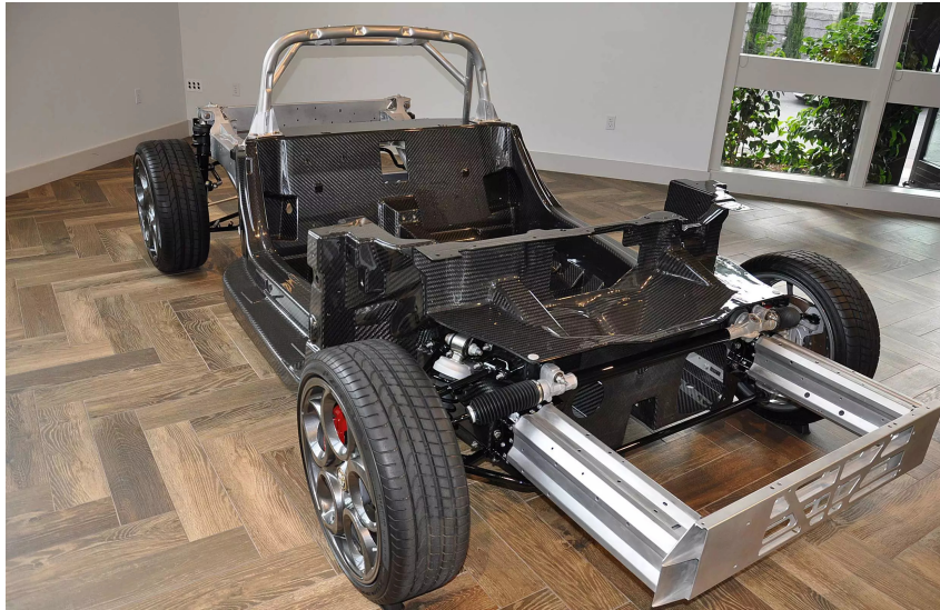
Fig. 1.1 Alfa Romeo 4C monocoque made of carbon fiber composites 1
