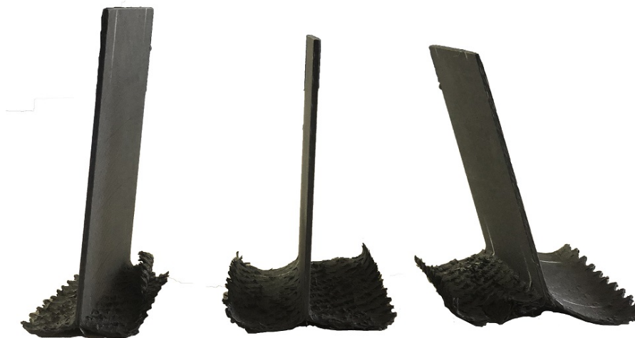
Fig. 4.14 Samples crushed under impact mass of 50 \text{ kg} and different velocities. From left to right: 4.69 \text{ m/s} ( 550 \text{ J} ), 5.29 \text{ m/s} ( 700 \text{ J} ), and 5.83 \text{ m/s} ( 850 \text{ J} ).
