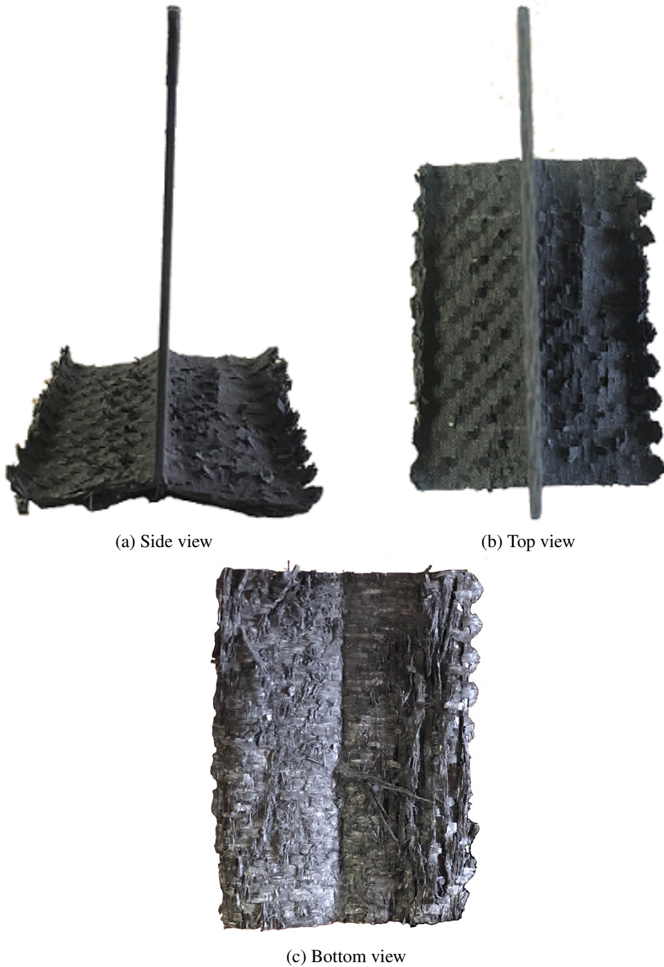
Fig. 4.16 Images of CFRP element after being crushed under impact energy of 850 J from different angles. Side and top views show the symmetrical crushing of element by not intervening with the newly developed fixture. The bottom view image shows the delamination in the middle of the element and fragmented parts of the inner layers.
