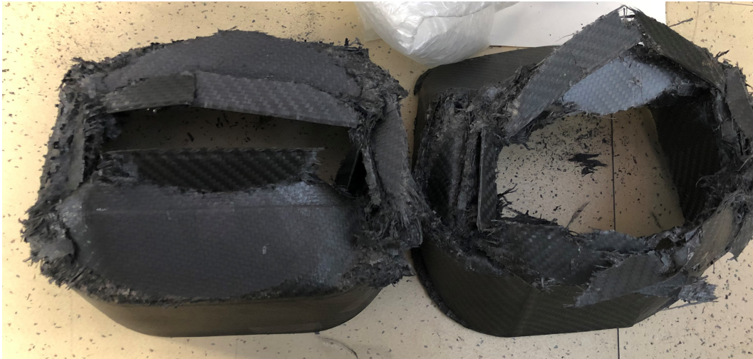
Fig. 4.22 Crushed CFRP components after quasi-static tests performed at 10 \text{ mm/min} rate.
