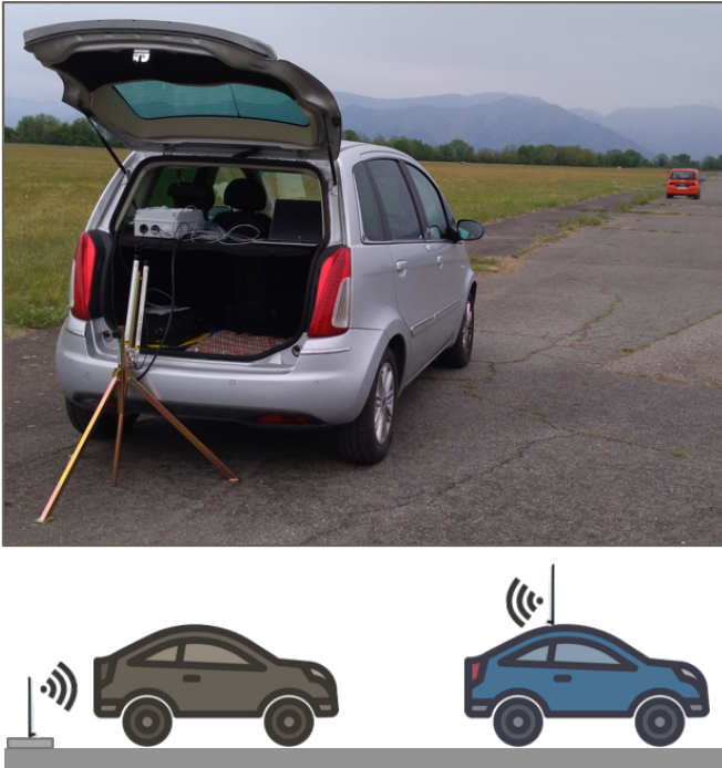
Figure 1: Test setup for measurements under NLOS conditions.
