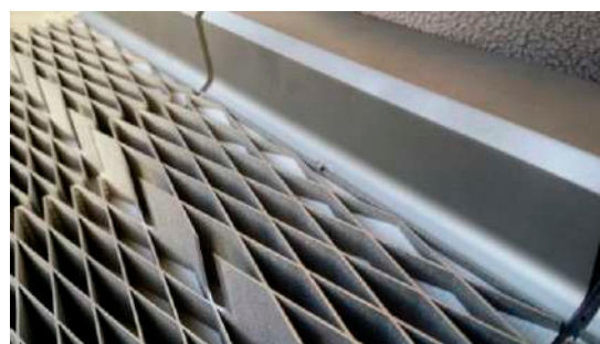
Figure 16. Test Article (TA) stator land with R3 rhomboidal cells.
