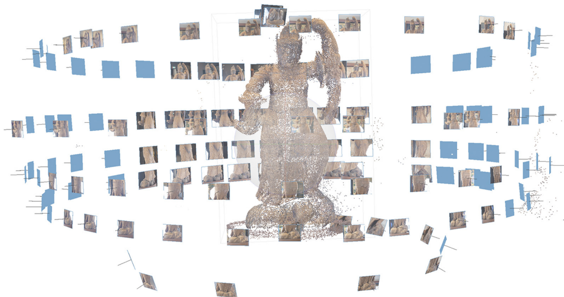
Figure 2. Photo alignment with sparse cloud. Processing: F. Ronco, S. Tamantini.
