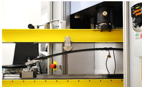
Figure 2.10 – Test configuration for the Leaf Spring component: Bending load
