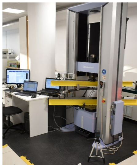
Figure 3.13 – Special fixture for Bending test of Leaf Spring mounted on Shimadzu dynamometer
