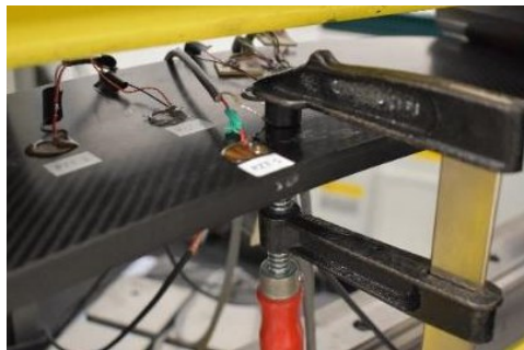
Figure 2.16 – Detail of the manual clamp applied in the case of Leaf Spring component
