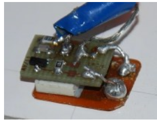
Figure 1.25 – Customized piezo amplifier for special SHM applications [23]
