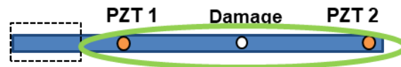
Figure 5.6 – Piezo couple PZT 1-2 studied for the influence of Damage on the Beam specimen
