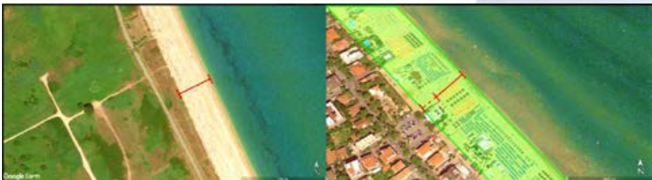
Fig. 1. Comparison between a natural coastal area in Abruzzo (Italy), and an anthropized sand beach that is located just a few km southward. The left panel shows the distance between the foredune and the shoreline (red line), whereas the right panel indicates approximately the area that should have been left natural to benefit from the protection of coastal dunes (green). The width (red line) of this area is the sum of two terms. The former (solid line) is the distance between the foredune and the shoreline and it is provided by the model. The latter (dotted line) is the foredune width, which is a function of the former distance.
