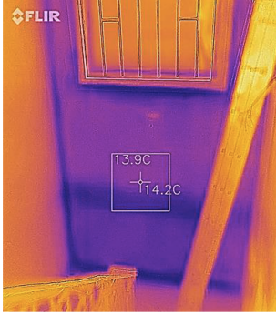
Fig. 2. Thermography of an external wall before the nanotechnology-based insulation.
