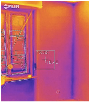
Fig. 3. Thermography of an external wall after the nanotechnology-based insulation.
