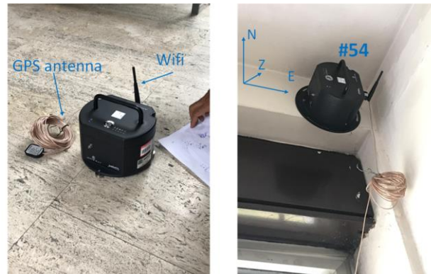
Figure 6 Force balance accelerometer for ambient vibration tests (#54 for C1 configuration).
