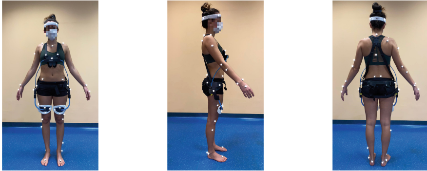
Fig. 2. Frontal, lateral, back views of female subject wearing the Laevo with passive markers.
