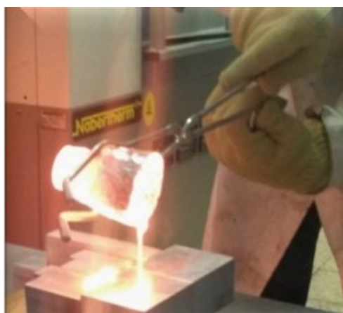
Fig. 2.15. Casting from a Pt/Rh crucible.
