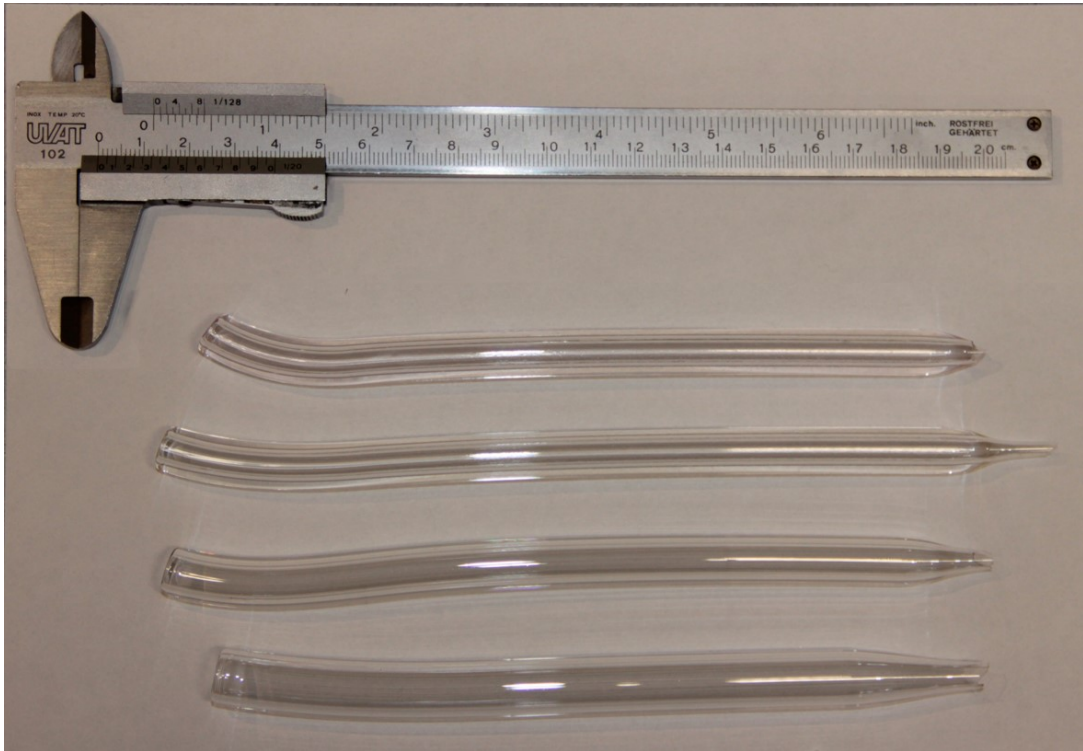
Fig. 5.20. Examples of some bioresorbable glass extruded tubes.
