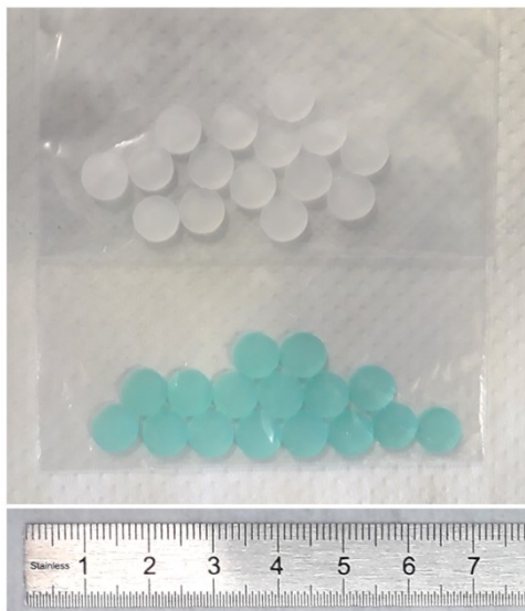
Fig. 6.9. Disk-shaped samples of undoped (white) and Cu-doped (bluish) glasses, obtained by slicing glass rods.
