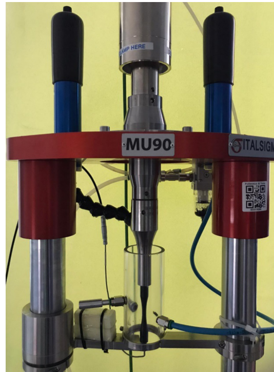
Figure 1. Ultrasonic fatigue testing machine MU90.
