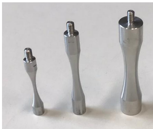
Figure 2. The three different investigated hourglass-specimens.
