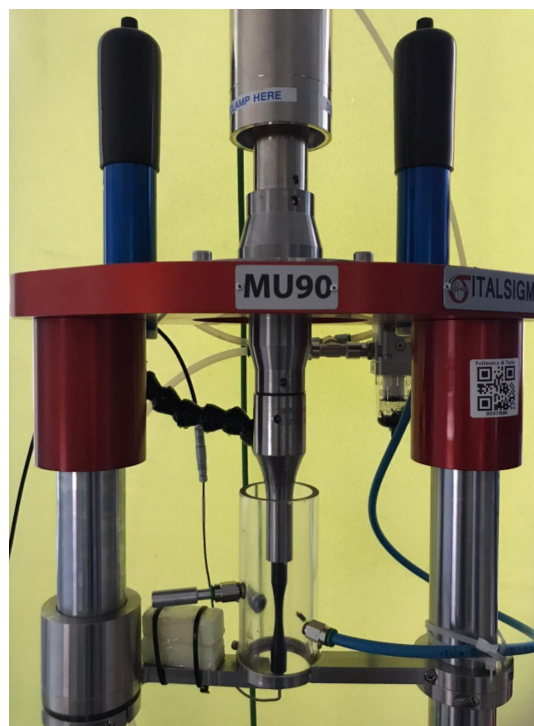
Figure 1. Ultrasonic fatigue testing machine MU90.
