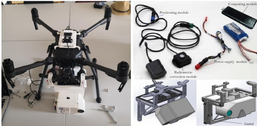
Figure 14. DJI Matrice 210 v2 configuration.
