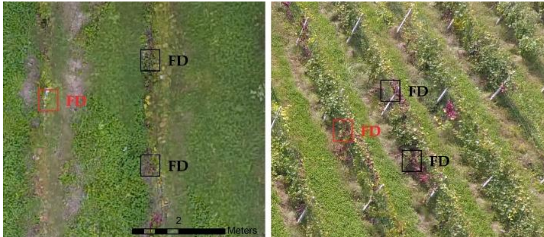
Figure 65. The influence of geometric artefacts, background homogeneity and the nadiral point of view. The comparison between an orthomosaic patch (on the left), and an original oblique image (on the right) in a vineyard [269].
