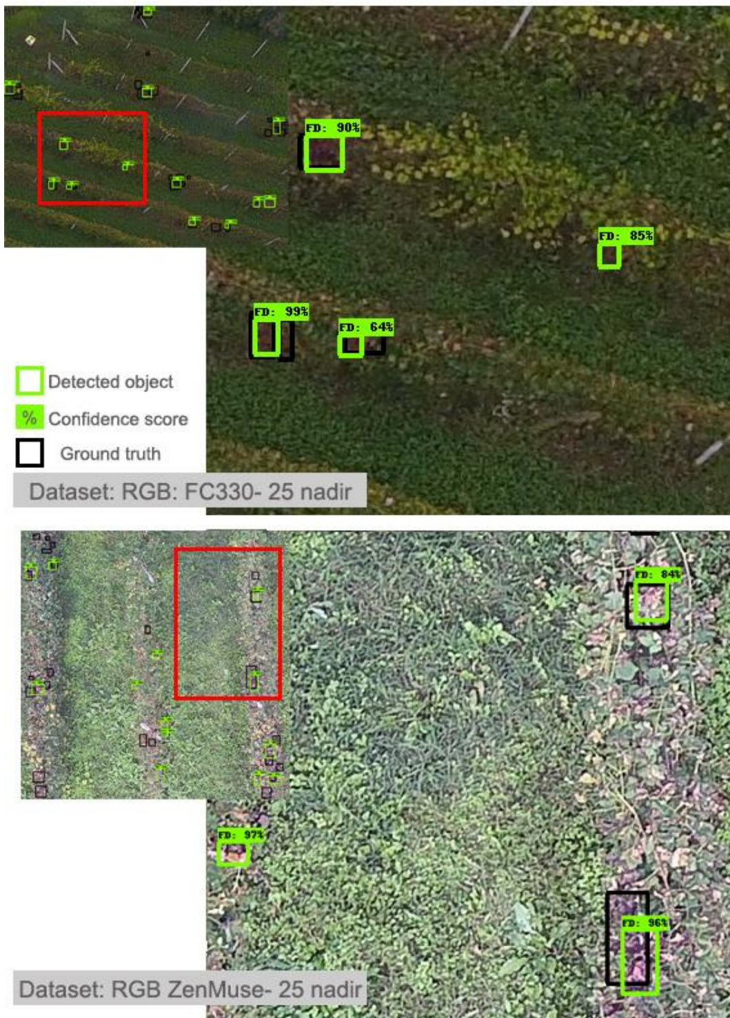
Figure 75. Faster R-CNN_ResNet 101 (test 4). Results of different types of images. In black, the reference data and in green detected diseased area.
