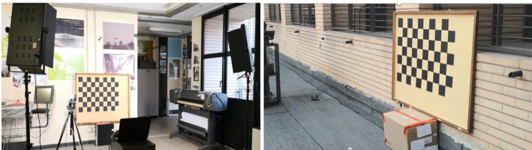
Figure 22. The acquisition set in an indoor environment, considering controlled illumination and exposure values (on the left), and in an outdoor environment (on the right). The calibration panel is a chessboard with an internal array of black and white squares (size of 10 cm).
