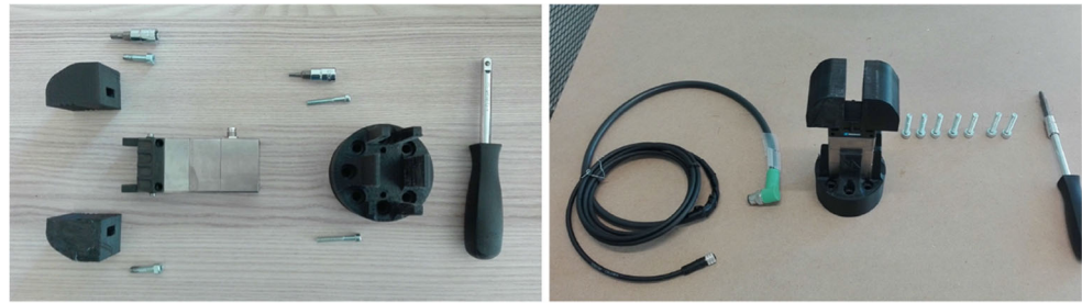
Fig. 6 Schunk's EGP 40-N-N-B gripping system with custom fingers and connection flange disassembled (left), and ready to be mounted (right)
