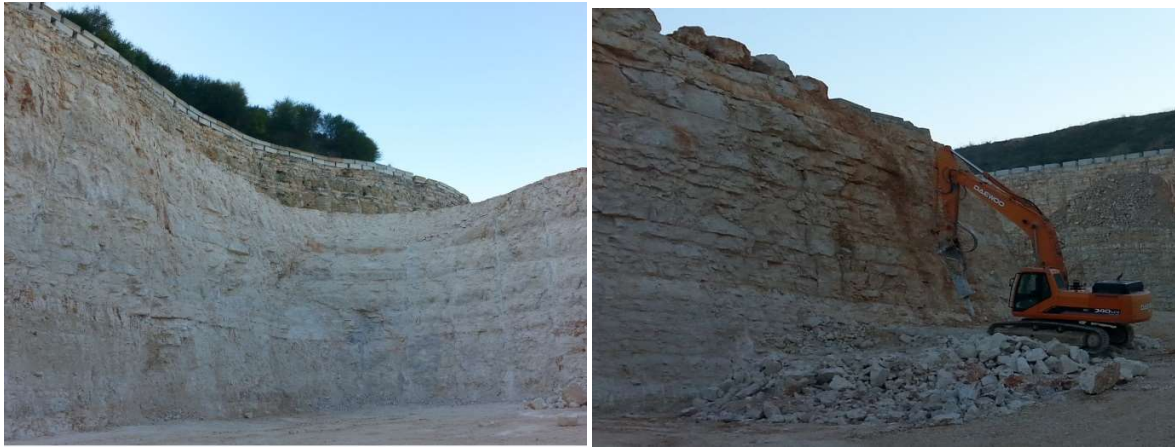
Figure 5. Quarry in limestone for aggregates, with two main joint sets; it is relevant the sub-horizontal system, with spacing of about 0.3–0.5 m. Left: blasting profile and few residual blast-holes in a vertical face 15 m high. Right: mechanical action of a hammer for detachment and scaling in a sub-vertical face 9 m high; scaling can represent an auxiliary procedure to solve mixed conditions (credits C. Oggeri and I. Cassone, quarry in South Italy).
