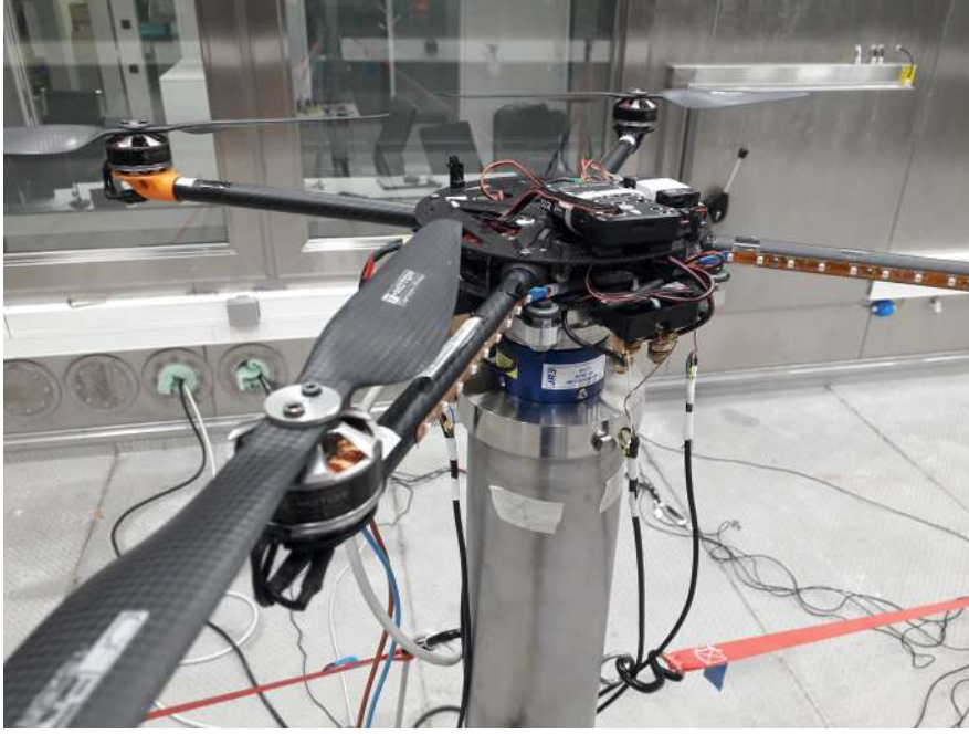
Figure 4.8: Q4L UAS and test stand during full vehicle test
