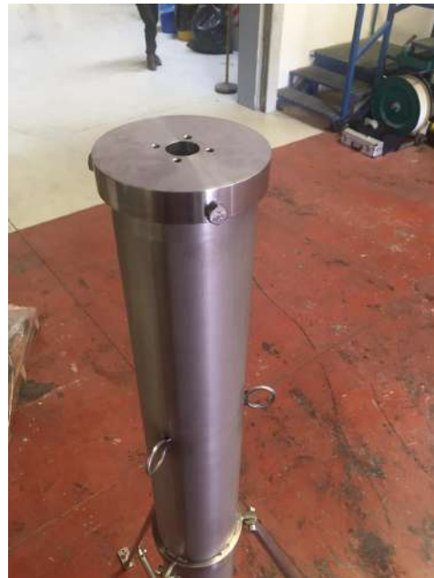
(b) Upper plate for load cell installation
