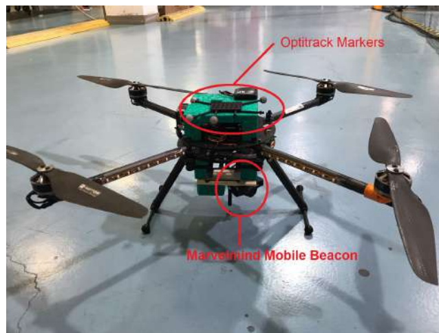
Figure D.10: UAS with Marvelmind beacon and optical marker for motion tracking
