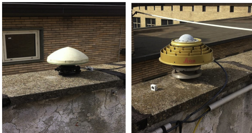
Fig. 4. Rover antenna (right) and master antenna (left).
