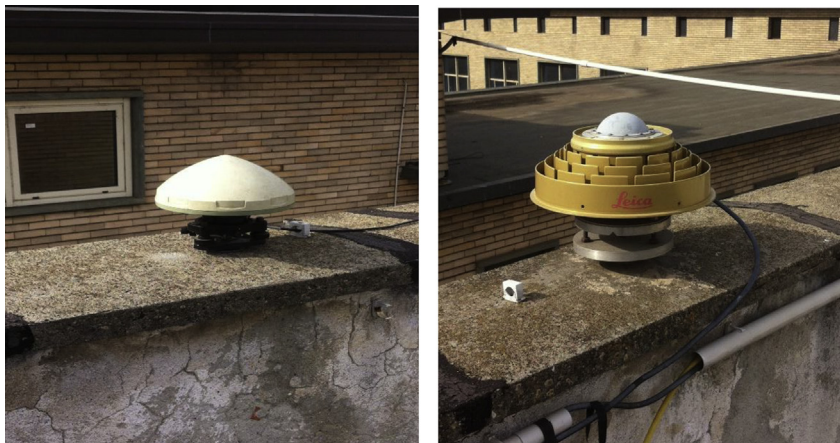
Fig. 4. Rover antenna (right) and master antenna (left).
