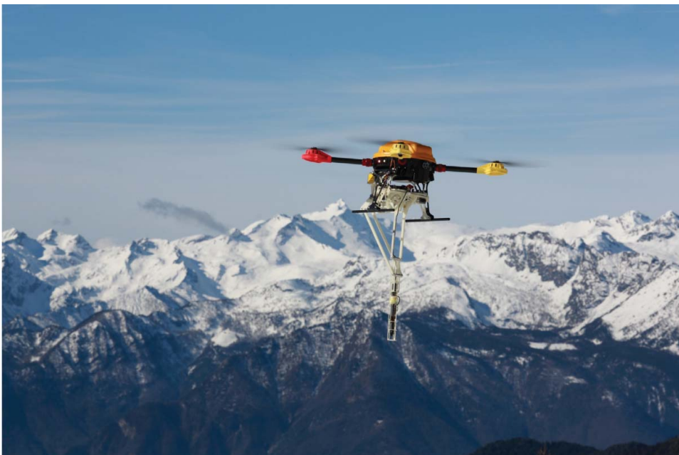
Figure 10. UAV during a search and rescue mission with avalanche beacon antenna deployed.
