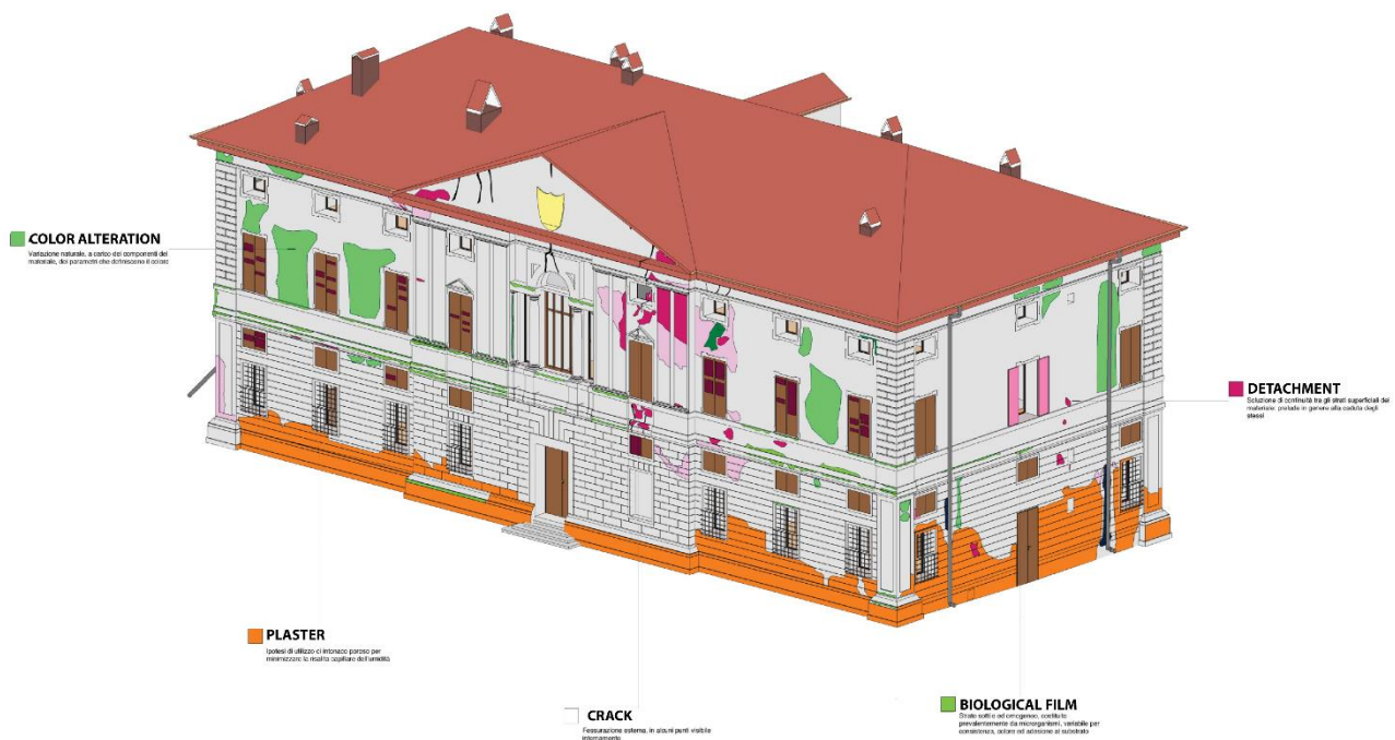
Figure 15. 3D visualization of the parametric model of Villa Sarmoris with the mapped decay.
