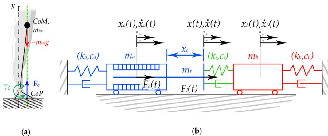
**Figure 2.** (a) Human body's reaction to low balance disturbances; (b) model of the system during strike phase for control application: actuator (in blue), interface (in green), target body (in red), state and measured variables (in black).
