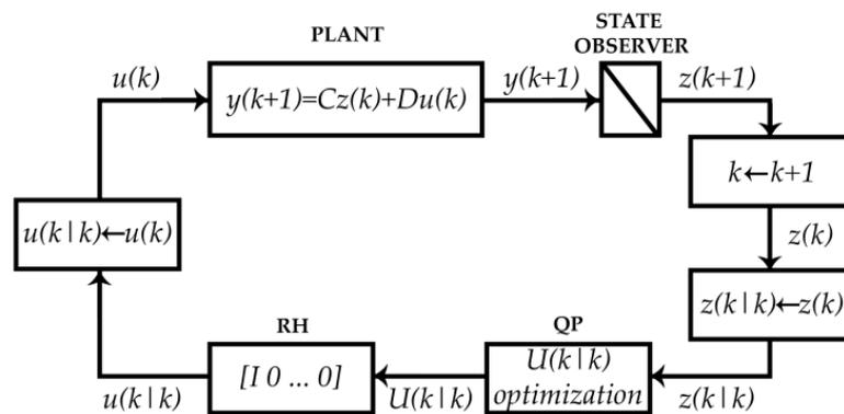
**Figure 3.** MPC algorithm loop and plant interaction.
