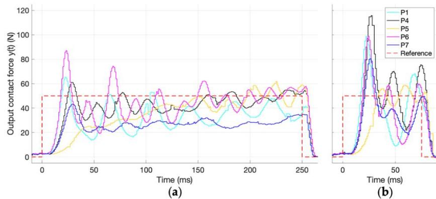
**Figure 5.** Force tracking of the MPC algorithm for the HIL: (a) refers to the R1 reference signal (50 N, 250 ms), (b) refers to the R2 reference signal (50 N, 75 ms). Reference force signal in red dashed lines, continuous lines refer to the output contact force obtained for different control parameters (see Table 5).
