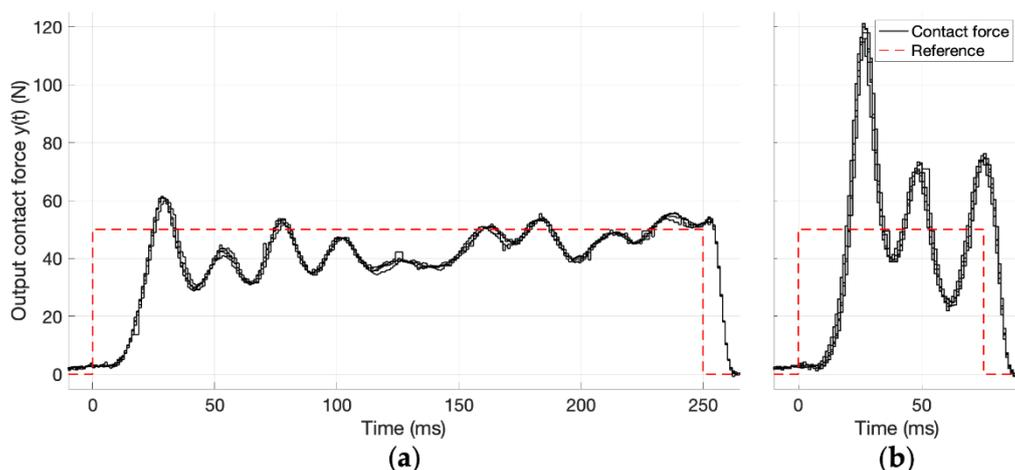
**Figure 6.** Force tracking of the MPC algorithm for the HIL: (a) refers to the R1 reference signal (50 N, 250 ms), (b) refers to the R2 reference signal (50 N, 75 ms). Reference force signal in red dashed lines, continuous lines refer to five consecutive force signals obtained for a particular selection of control parameters (see Table 5, P4 profile).
