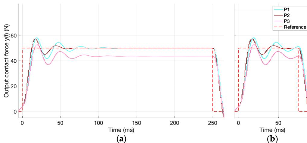
**Figure 4.** Force tracking of the MPC algorithm for the MIL: (a) refers to the R1 reference signal (50 N, 250 ms), (b) refers to the R2 reference signal (50 N, 75 ms). Reference force signal in red dashed lines, continuous lines refer to the output contact force obtained for different control parameters (see Table 4).
