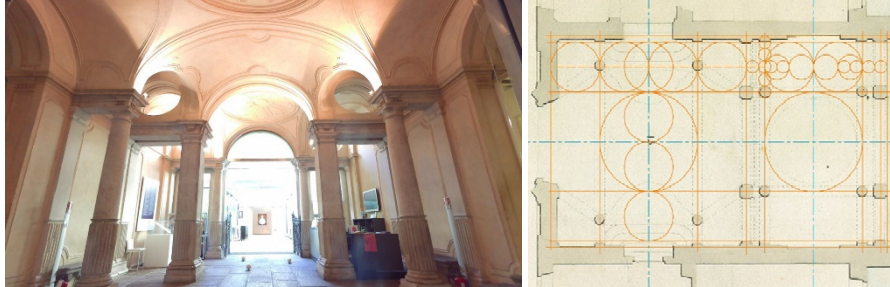
Fig. 1. Atrium of Palazzo Mazzonis in Turin; excerpt of the survey drawing dated 1st July 1845 with superimposition of graphical analysis. Source: Archivio Storico del Comune di Torino, Tipi e dis., cart. 63, fasc. 9, dis. 1, tav III. Photo: F. Natta. Graphic processing: F. Ronco.
