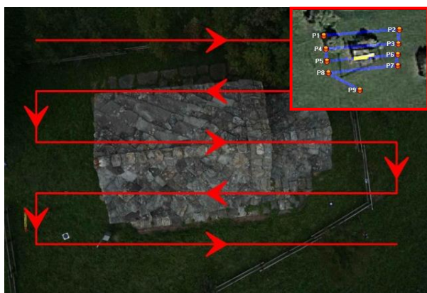
Figure 4. Schema of the linear flight-plan for the acquisition of the nadir images (a screenshot of the Mikrokopter tool is in the top right part of the image)
