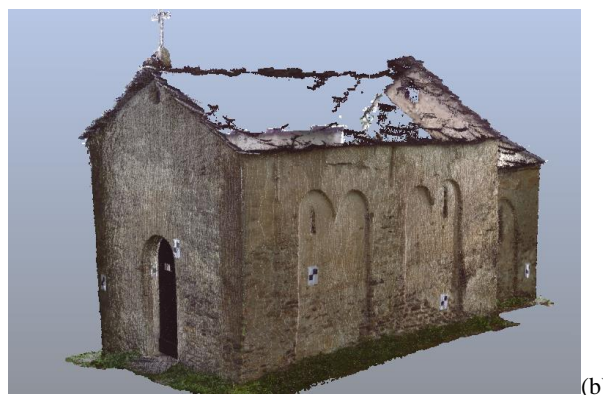
Figure 8. Original TLS point cloud (a), cleaned TLS point cloud of the Chapel (b)
