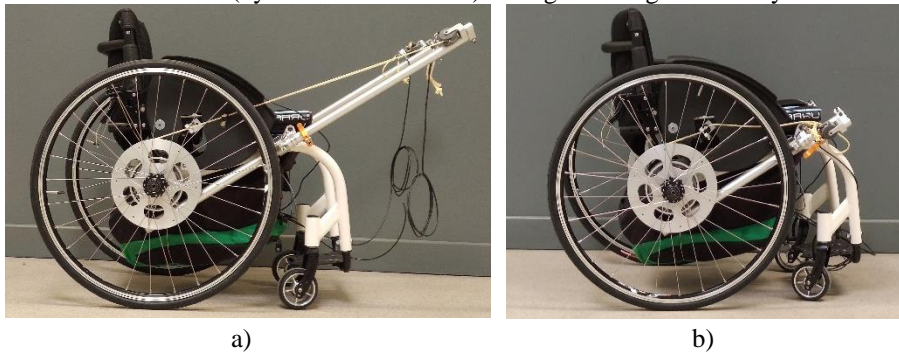
Fig. 3. a) Innovative configuration and b) with retracted telescopic rod
