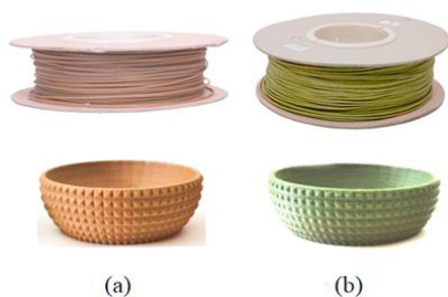
Fig. 2. Thermoplastic bio-composite filaments: (a) HEMP; (b) WEED.
