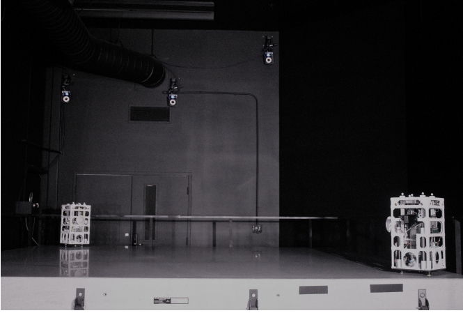
Fig. 2. NPS-POSEIDYN testbed with the Vicon motion capture cameras, FSSs, and granite monolith in the Spacecraft Robotics Laboratory at the Naval Postgraduate School. The target FSS is on the right and the chaser FSS is on the left. For obvious reasons, the applicability of the testbed, as a high-fidelity dynamic simulator, is limited to short lived close proximity operations, with respect to the planar motion only.
