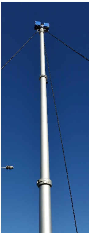
Figure 8: Telescopic pole equipping the Faro laser scanner during the case study 3D survey.
