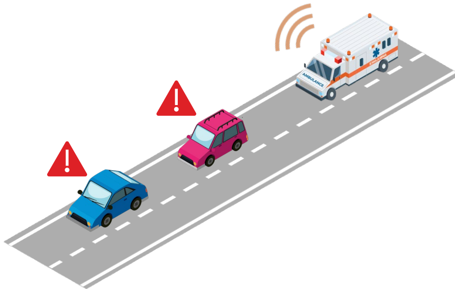
(b) An example of a real implementation of the Emergency Vehicle Alert application, with an ambulance transmitting DENMs to inform vehicles about its presence.
