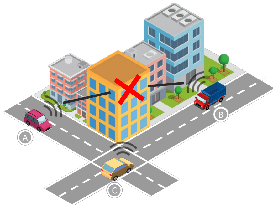
Figure 4.11: Typical situation in which the silent version of CAS does not identify a collision: vehicles A and B are going to collide, but the building in the middle attenuate their radio connection. Vehicle C does not help, because DENM transmission is disabled.
