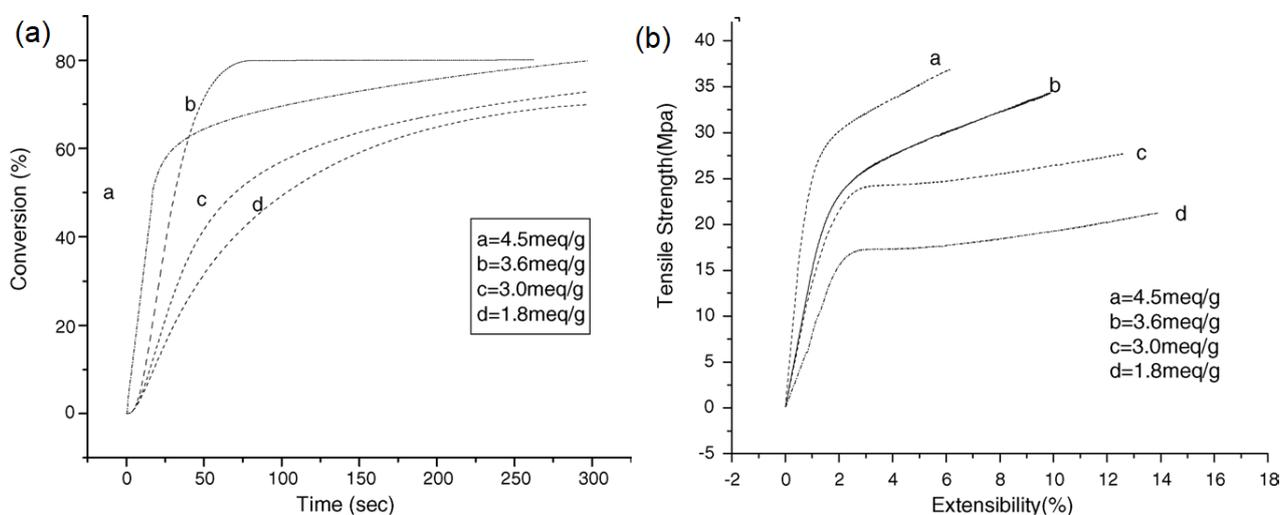
**Figure 4.** (a) Conversion comparison for samples containing different C=C contents, using 4% Darocur 2959 and 80 mW·cm<sup>-2</sup> light intensity. (b) Stress-strain curves of UV-cured waterborne
