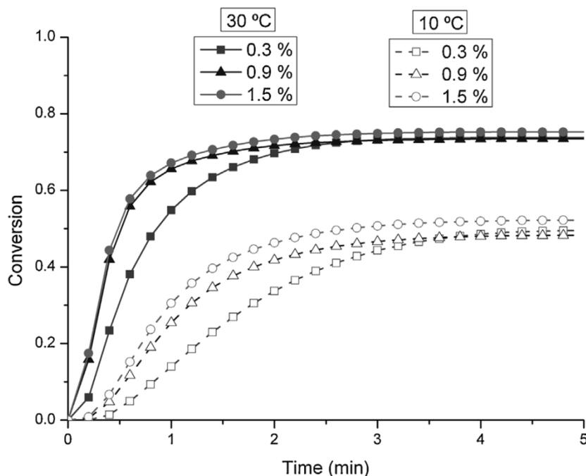
**Figure 9.** Curing conversion of UV-WPU sample at 10 and 30 °C, using different photoinitiator amounts [32]. Reproduced with permission from Ref. 31, Llorente O, *et al.* (2016) *Prog Org Coat* 99:437–442. Copyright © 2016 Elsevier B.V.
