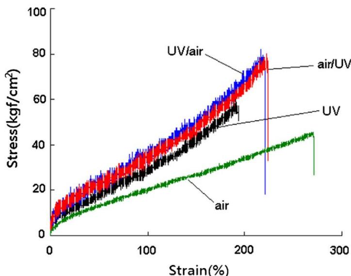
**Figure 10.** Stress-strain curves of UV-WPU coatings prepared using different curing processes [138]. Reproduced with permission from Ref. 137, Chang, *et al* (2013) *Prog Org Coat* 76(7-8):1024–1031. Copyright © 2013 Elsevier B.V.
