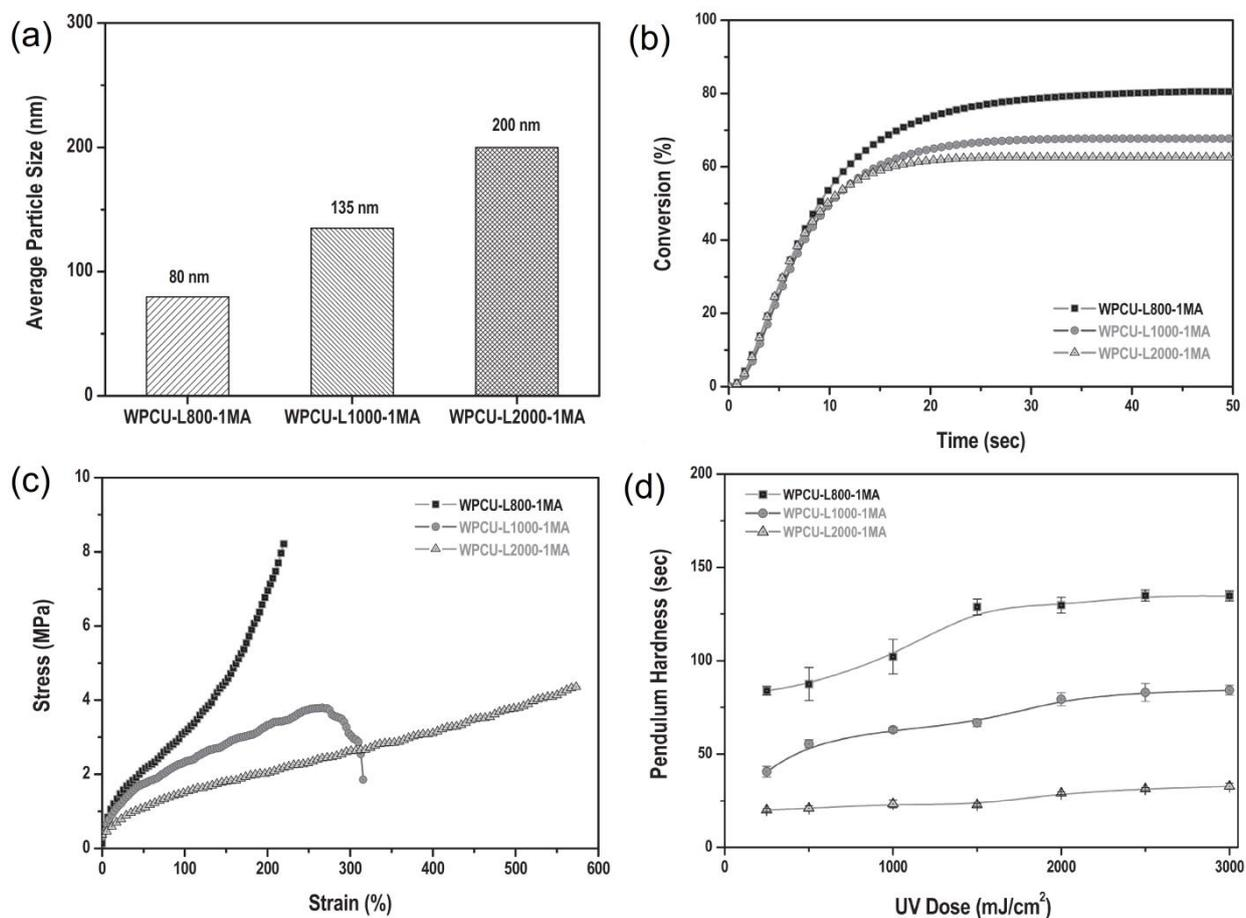
**Figure 3.** Effect of molar mass on the properties of a coating synthesized using different PCDs ((■) 800 g/mol; (●) 1000 g/mol; (▲) 2000 g/mol). (a) Average particle size of the dispersion. (b) C=C double bond conversion vs. time by photo-DSC. (c) Tensile behavior of the cured film. (d) Pendulum hardness of the cured film as function of the UV-dose [24]. Adapted with permission from Ref. 23, Hwang HD, *et al.* (2011) *Prog Org Coat* 72:663–675. Copyright © 2011 by Elsevier B.V.
