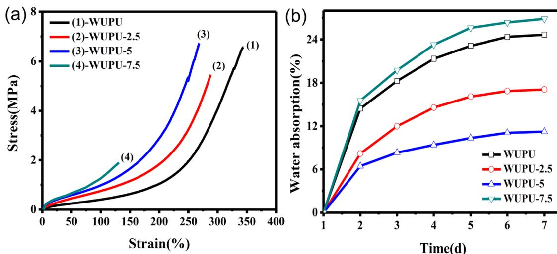
**Figure 6.** (a) Tensile behavior and (b) water absorption of APTES-HEA-WPU films. WUPU-x, where x is the mass weight fraction of the APTES-HEA [51]. Adapted with permission from Ref. 50, Zhang S, *et al.* (2015) *Colloids Surf A Physicochem Eng Asp* 468:1–9. Copyright © 2014 Elsevier B.V.
