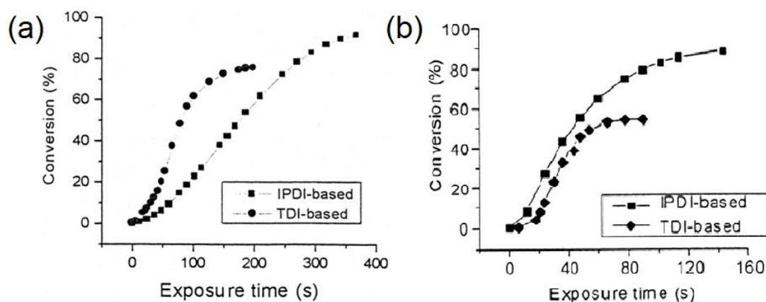
**Figure 2.** (a) Effect of diisocyanate type on curing kinetics of chain-extended UV-WPU from PEG 400 g/mol and (b) Effect of diisocyanate type on curing kinetics of chain-extended UV-WPU from PEG 2000 g/mol [92]. Adapted with permission from Ref. 91, Yang J, *et al.* (2002) *J Appl Polym Sci* 84:1818–1831. Copyright © 2002 Wiley Periodicals, Inc.
