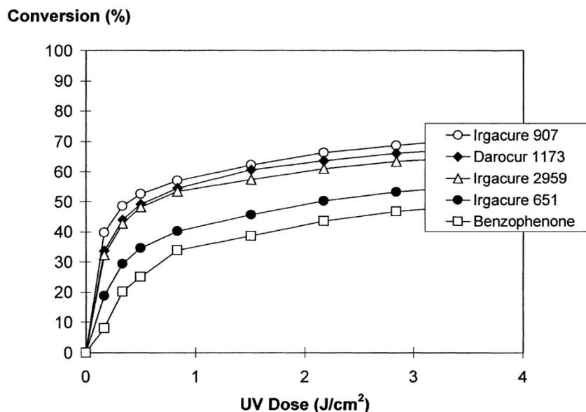
**Figure 8.** Influence of the photoinitiator on the UV-curing of a WPU coating. Temperature: 25°C; light intensity=60 mW/cm<sup>-2</sup>; [photoinitiator]=1 wt.% [165]. Reproduced with permission from Ref. 164, Masson F, *et al.* (2000) *Prog Org Coat* 39(2–4) 115–126. Copyright © 2000 Elsevier Science S.A
