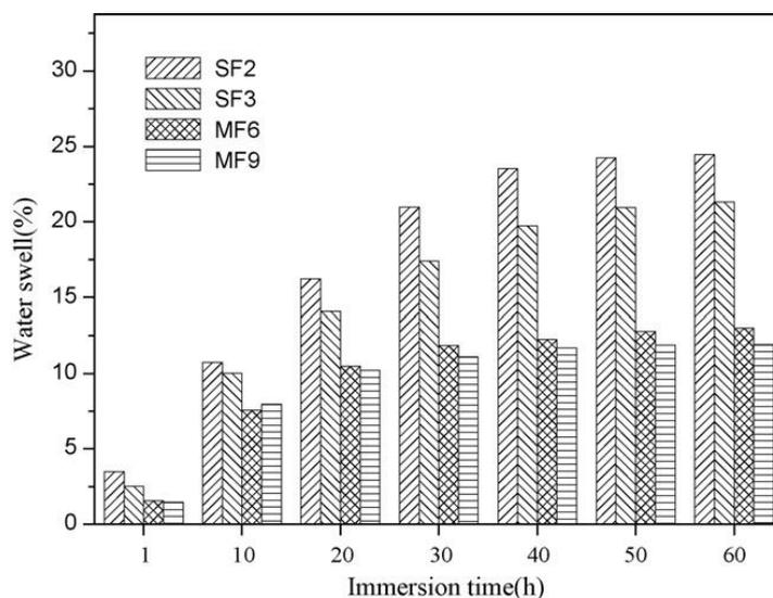
**Figure 5.** Water swell percentage *versus* immersion time for UV-WPU films with different C=C contents [6]. Reproduced with permission from Ref. 5, Zhang T, *et al.* (2010) *Prog Org Coat* 68:201-207. Copyright © 2010 Elsevier B.V.
