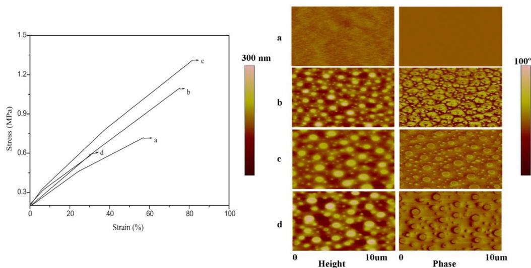
**Figure 7.** (a) Stress–strain curves for the hybrid films: (a) UV-WPU, (b) UV-WPU-Silica-5, (c) UV-WPU-Silica-10, (d) UV-WPU-Silica-15; (b) AFM images of topography (left) and phase (right) for: (a) UV-WPU, (b) UV-WPU-Silica -5, (c) UV-WPU-Silica -10, (d) UV-WPU-Silica-15 [88]. Adapted with permission from Ref. 87, S. Zhang S, *et al.* (2011) *Prog Org Coat* 70:1–8. Copyright © 2010 Elsevier B.V.
