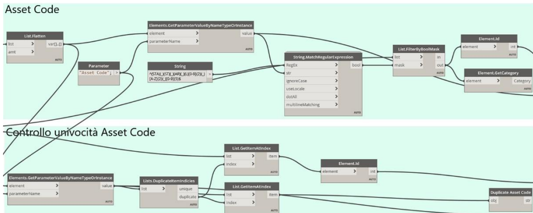
Figure 85 – Example of a substantial check in Autodesk Dynamo
