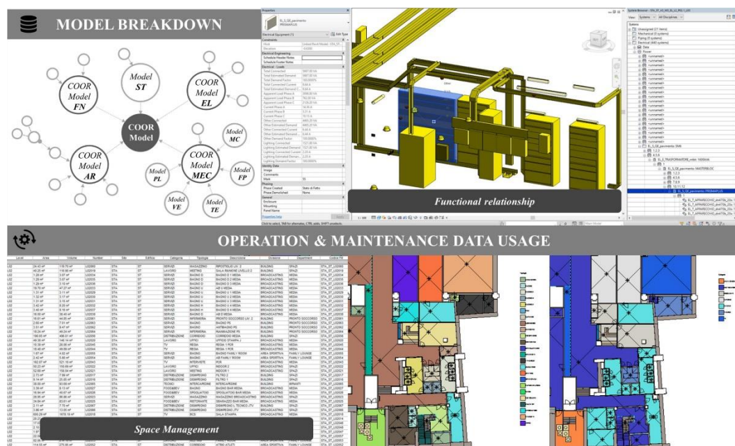
Figure 20 – Uses of an As-is model for FM (Barbero, Del Giudice, Ugliotti, & Osello, 2020).
