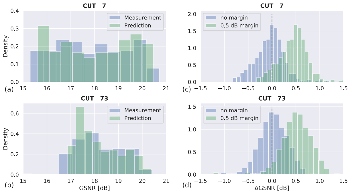
FIGURE 12. The measured and predicted GSNR power distributions for: (a) CUT 7 and (b) CUT 73, along with the corresponding \Delta GSNR power distributions with and without a 0.5 dB margin for: (c) CUT 7 and (d) CUT 73.
