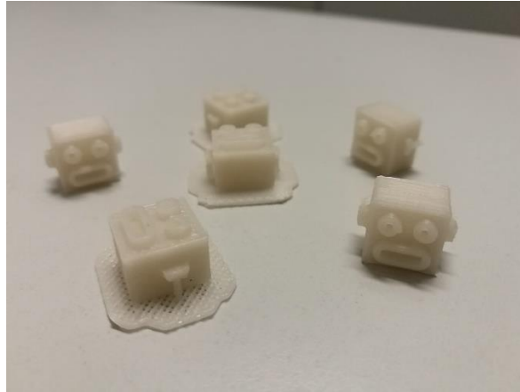
Figure 5. Robot-heads used as model parts for the printing tests.
