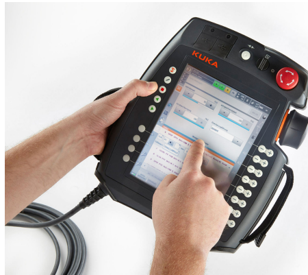
Figure 1: KUKA Smart Pad (SP): this is the device that is used by operators to manually control and program the robot. It incorporates a touch-based graphics interfaces, as well as some physical buttons and switches for safety-critical operations.
