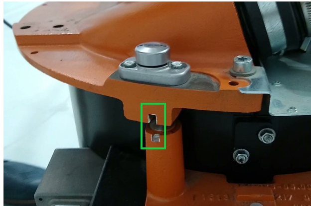
Figure 2: Axis #1 of a KUKA KR-16 robot in pre-calibration position. The green box highlights the visual references to be aligned by the operator in the first step of the MP.
